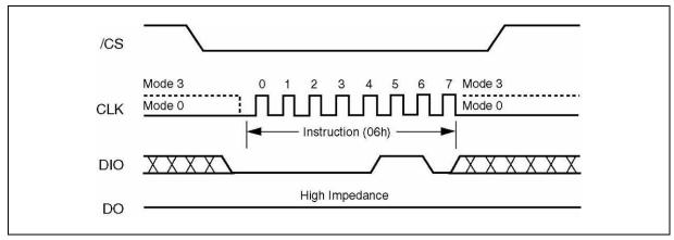
Figure 4. Write Enable Instruction Sequence Diagram
