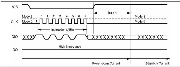
Figure 17. Release Power-down Instruction Sequence
