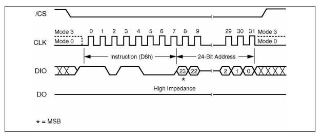
Figure 14. Block Erase Instruction Sequence Diagram
