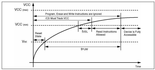
Figure 21. Power-up Timing and Voltage Levels
