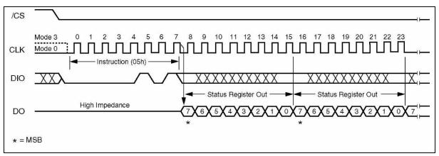
Figure 6. Read Status Register Instruction Sequence Diagram
