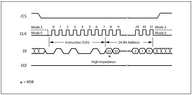
Figure 13. 32KB Block Erase Instruction Sequence Diagram
