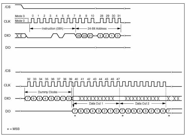
Figure 9. Fast Read Instruction Sequence Diagram
