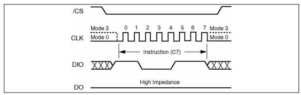
Figure 15. Chip Erase Instruction Sequence Diagram
