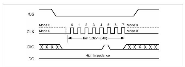
Figure 5. Write Disable Instruction Sequence Diagram
