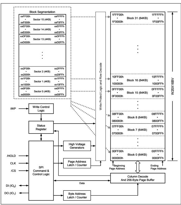
Figure 2. W25X16BV Block Diagram
