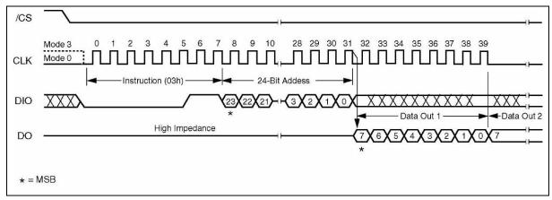
Figure 8. Read Data Instruction Sequence Diagram
