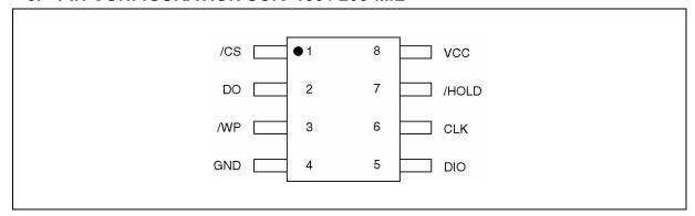
Figure 1a. W25X16BV Pin Assignments, 8-pin SOIC 150 / 208-mil (Package Code SN & SS)
