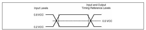
Figure 22. AC Measurement I/O Waveform
