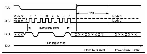
Figure 16. Deep Power-down Instruction Sequence Diagram
