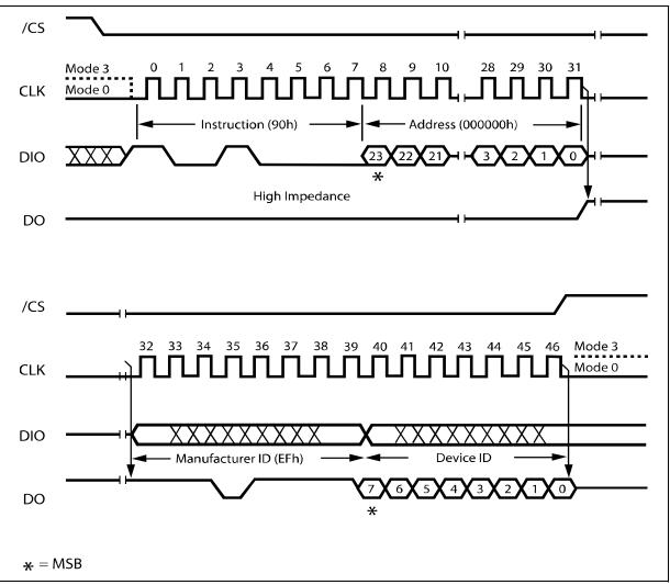
Figure 19. Read Manufacturer / Device ID Diagram
